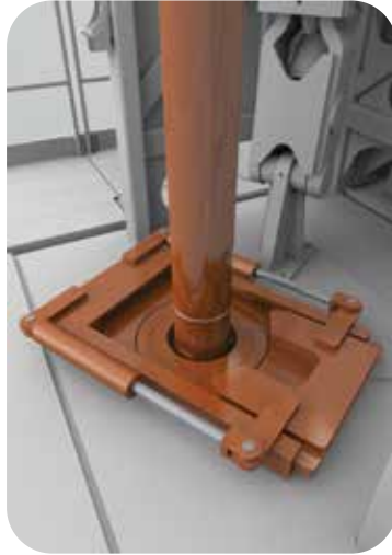
Align Drill Rod Flats With Fork
